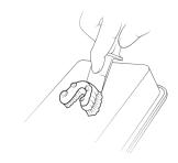
Remove the hybrid denture from the build platform
