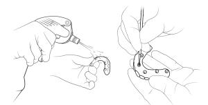
Use compressed air to remove final debris and evaporate any IPA that is trapped in the screw channels.
