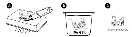
In total, the print should spend no more than **10 minutes** in alcohol to avoid microcracks and abrasions. Once cleaned, air-dry the print using compressed air. If the model feels tacky to the touch or has a shine, dunk it in IPA a few more times until the excess resin is totally removed.
