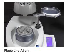
Place the model in the center of the base of the machine. Align plastic and heating element over the model.
